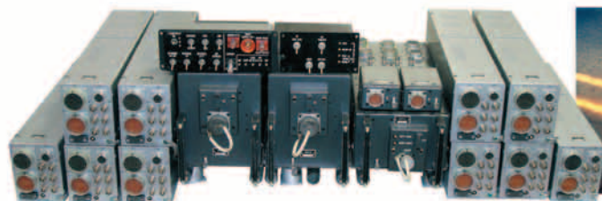
General view of stores management system
